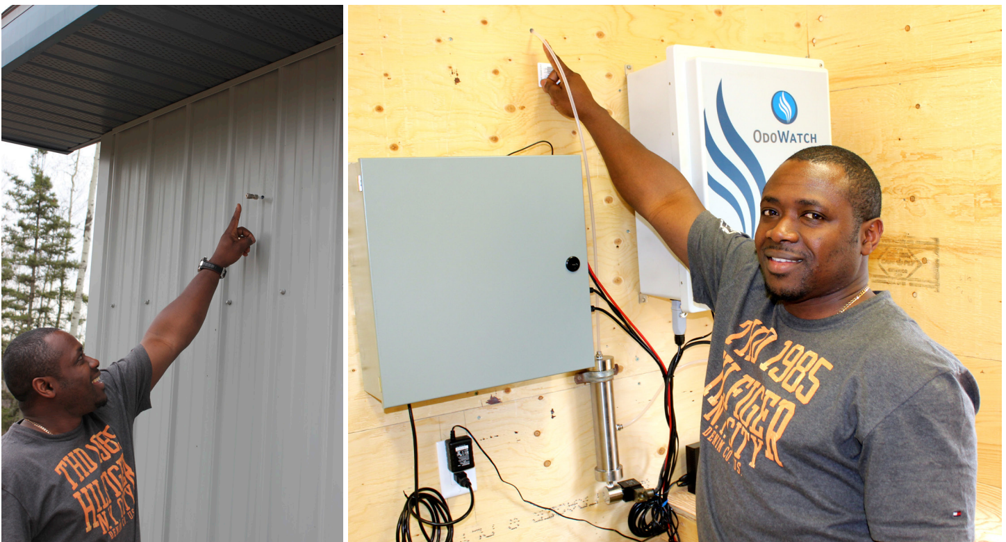
SNIFF SNIFF. Senior Environment Coordinator, Eddison Lee-Johnson points at an “E-Nose”, an electronic nose. The purpose of the E-Nose is to monitor odours in our air that may indicate pollutants.
